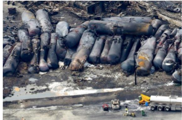
Explosive Trains. This photo shows the aftermath of a DOT-111 train derailment and subsequent explosion that brought crude oil into Lac-Mégantic, Québec. The explosion killed 47.
